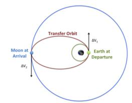
In the process of getting to the Moon, the engines perform a prograde (accelerating in the direction of travel) at a given point in the LEO (MoonConnection, 2016), to bring the apoapse, which is furthest point in orbit from Earth (Bruce, 2009), approximately 3 days ahead of the Moon's orbit. The velocity must be scaled up to over 11.2 kms<sup>-1</sup> order to bring the apoapse up sufficiently. Simply put, this is requires an additional
