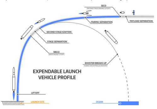
trajector. Launch profile of Falcon 9 (Gardi & Ross, 2016) sired altitude at which to circularise, the rocket will have to begin its gravity turn at a sufficient altitude. Because
